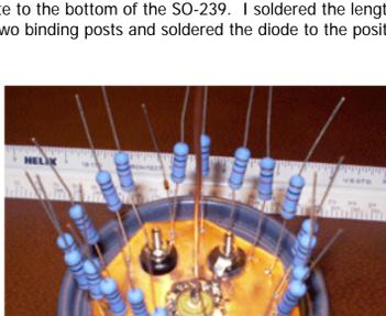
I added the bottom copper plate, using high temp silver solder. We are done and ready to fill with the mineral oil. (I did not trim the leads protruding through the bottom plate: again the more metal, the more heat will dissipate)
