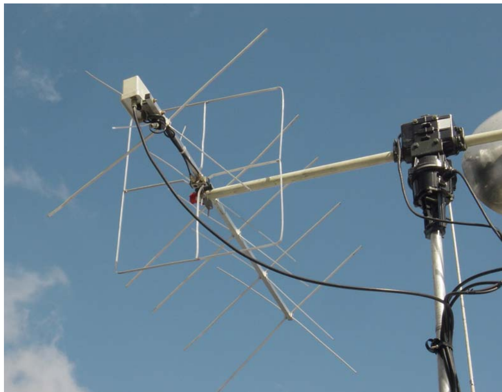
Fig 3. Isolated inputs of the new quad element
