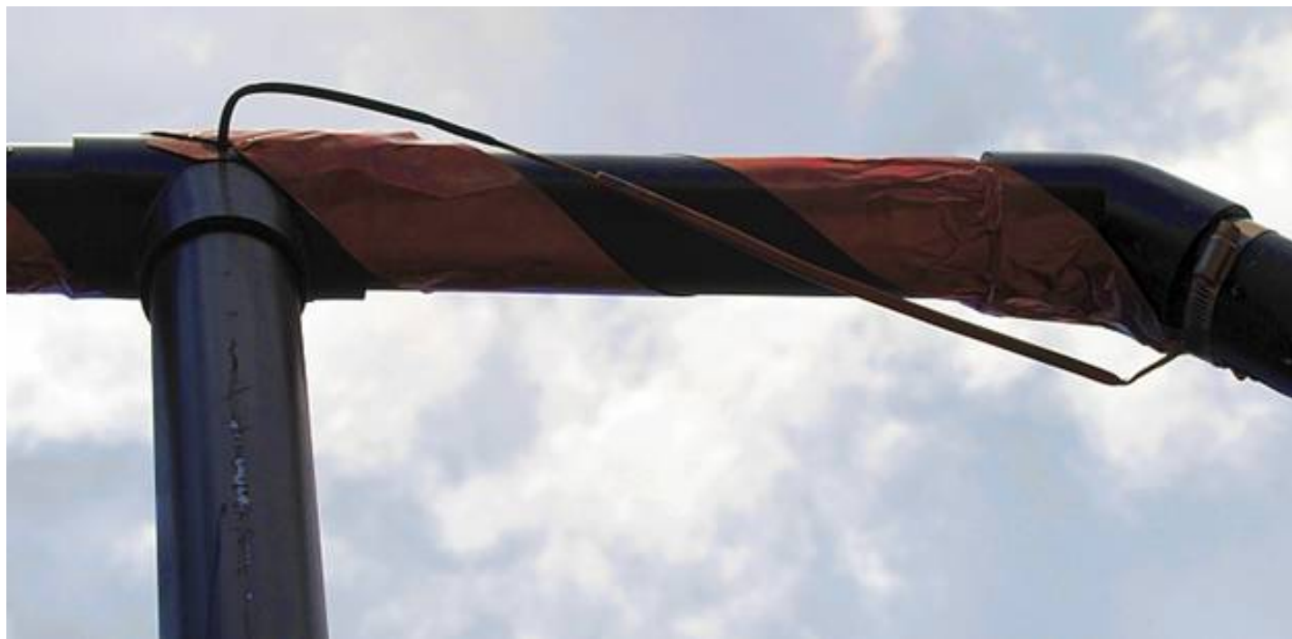
Rear view of gamma match in operating position, indicating how the SO-239 connection exits from the rear of the PVC T
