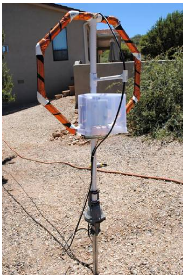
Finished 20 thru 10 meter loop ..... Just needs paint
