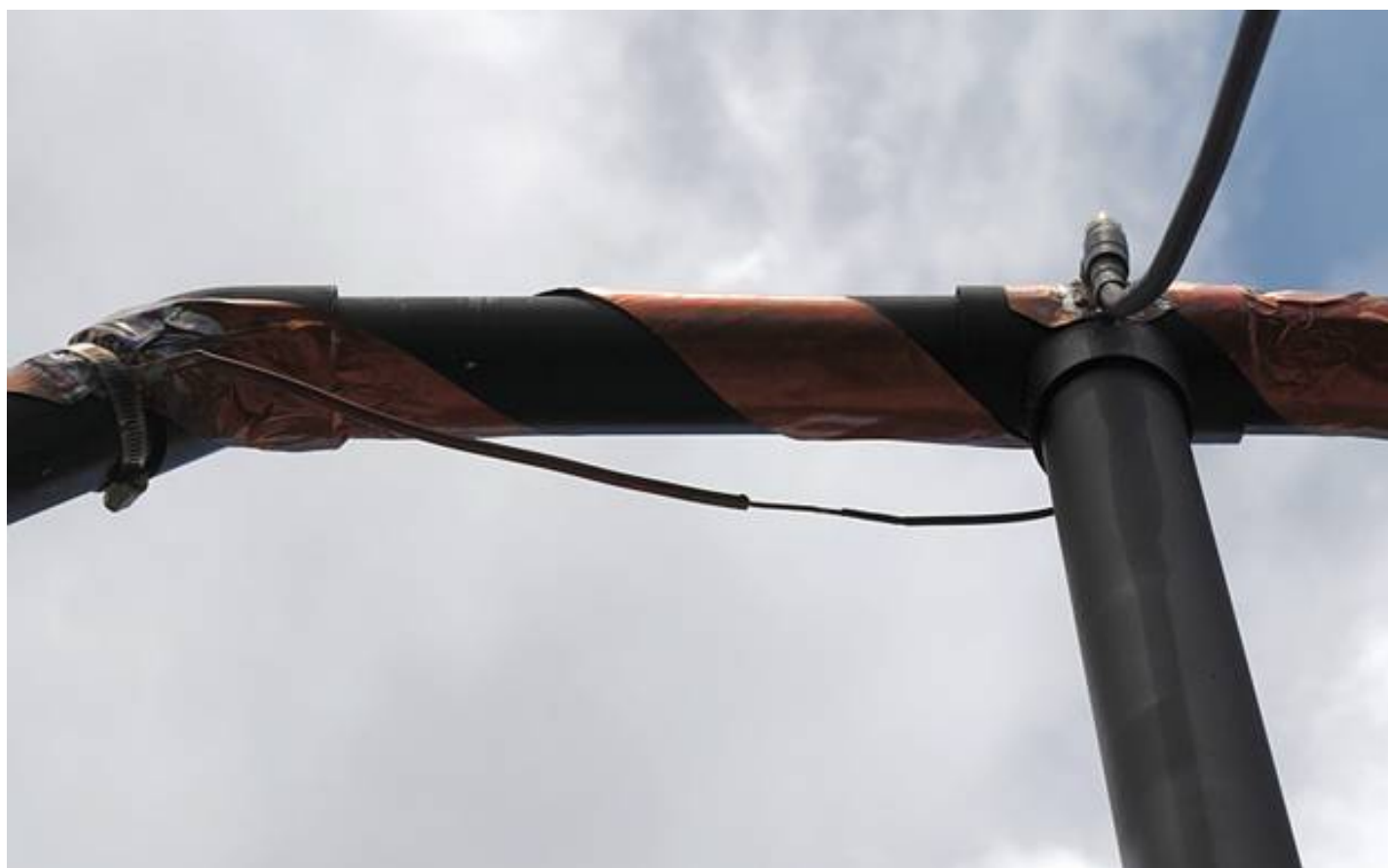
Front view of gamma match soldered in place; 1:1 @ 50 ohms
