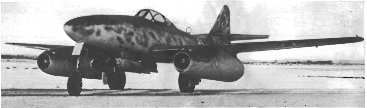
(Above and right) An Me 262A-2a Werk-Nr. 110 813 with two 551-lb. SC 250 bombs. This fighter-bomber variant, which first entered service with a detachment of KG 51 commanded by Major Wolfgang Schenck during the summer of 1944, differed from the standard fighter solely in having pylons and bomb-fusing equipment.
