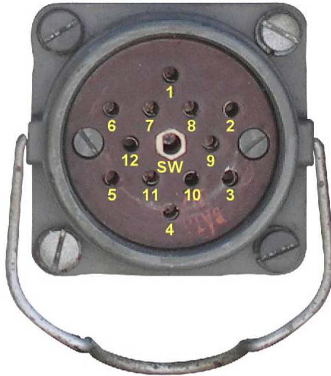
Optional 12-pin round connector on front panel of Amplifier & Interconnect Unit
