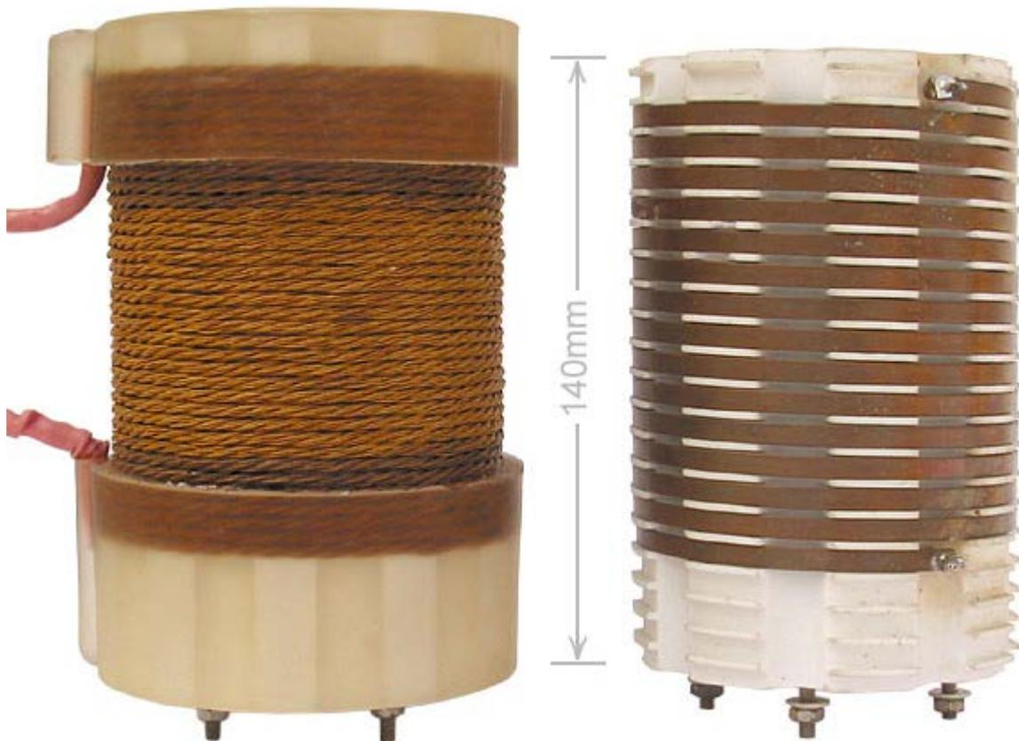
**Litzendraht coil and copper-strip coil** (Racal-BCC VRA549 automatic HF antenna tuner)
