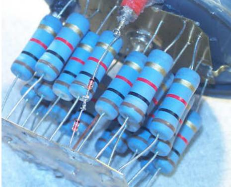
Next, we fill the quart paint can with mineral oil, which is a safe (You can actually drink it! - No PCB's for our dummy!), inexpensive, and readily available. The mineral oil works very well for conducting heat away from our resistors - It enables us to use 60W worth of resistors safely with a 130W rig.
