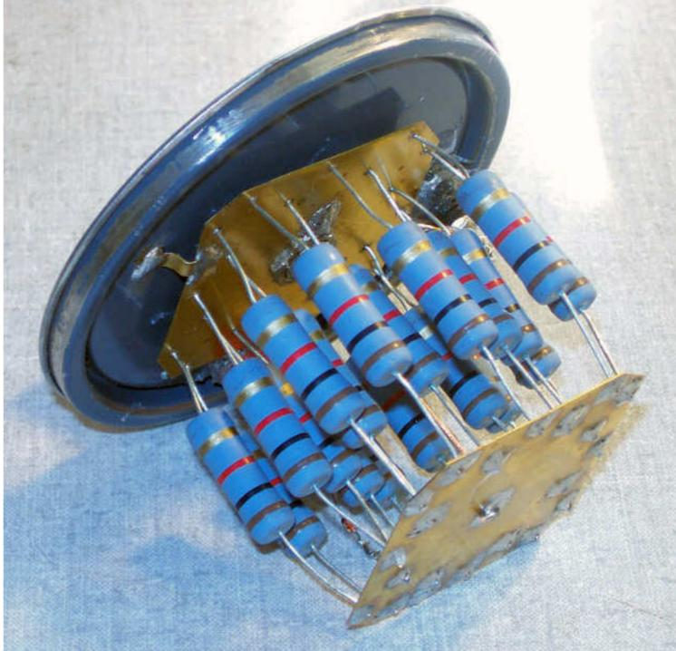
Here is another picture of the assembly, showing the connector and the optional binding posts. I used a BNC connector, but you probably want to use an SO-239.
