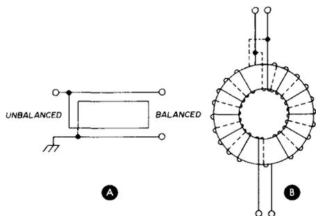
fig. 2. Circuit (A) and construction (B) of a 4:1 balun for use with the suitcase antenna. Although the author used a Mullard toroid core, an Amidon T-50-2 core with 10 or more bifilar windings of number-14 wire would be suitable.
