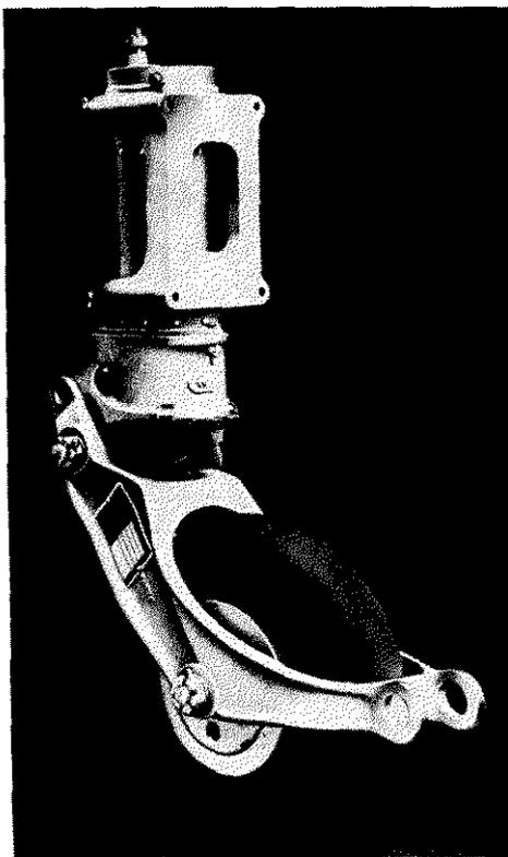
TAIL WHEEL ASSEMBLY (left) AND CONTROL COLUMN ASSEMBLY (below), INCORPORATING "ELEKTRON" MAGNESIUM CASTINGS, FOR USE IN AIRCRAFT
