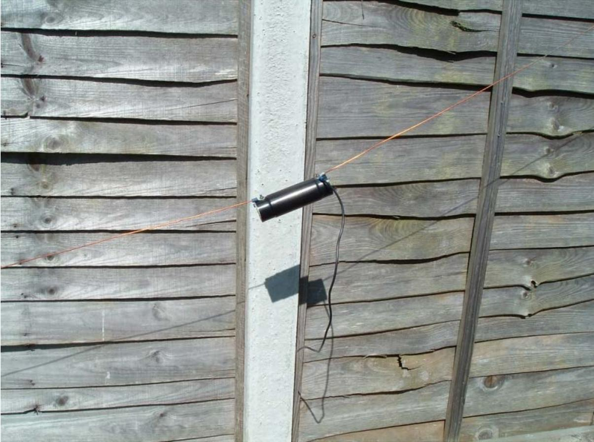
Here is the location to tune the 7 MHz (40m) section. When I first made the aerial, I miscalculated the amount of wire taken up by the threading through the feeder. To counteract this I added wire on the end and used this to tune the band.
