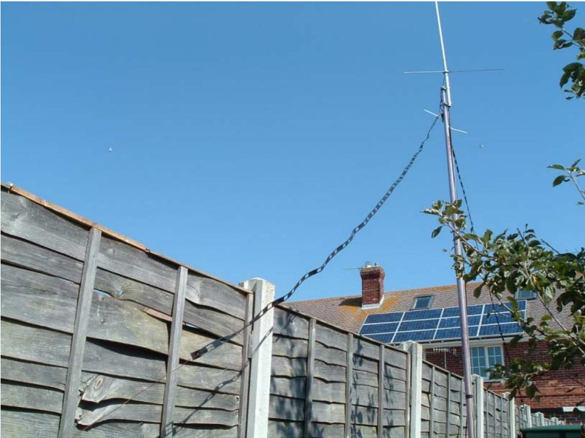
A image of one of the dipoles arms. It is made of 450 ohm open wire feeder with a single core wire threaded though the holes drilled in the spacers. The end of the feeder is soldered together and this is the location to tune the 14MHz (20m) section of the antenna. Trim feeder off and if you make a mistake just solder a single lenght of wire here and trim back again (a bit like the coil picture)
