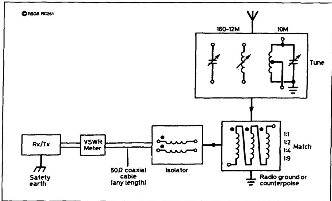
Figure 3. Layout of antenna to transmitter interface.
