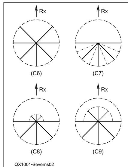
Figure 2 — Additional asymmetric ground systems.
