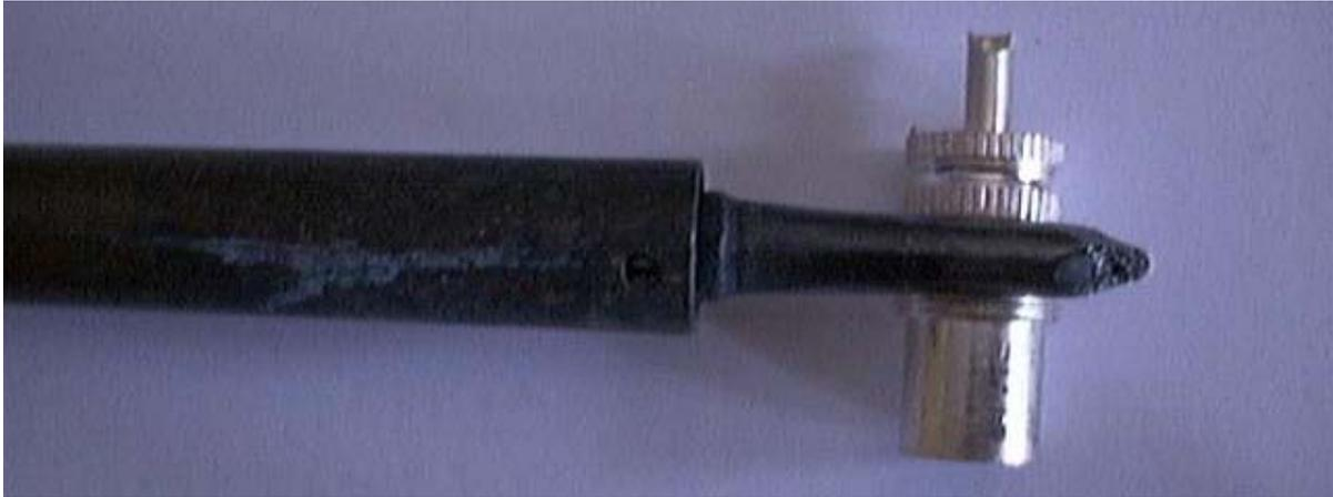
So we've got our coax prepped, our irons hot, and it's time to screw on the PL259. Remember slide the outer threaded barrel on to the coax first. I digress.
