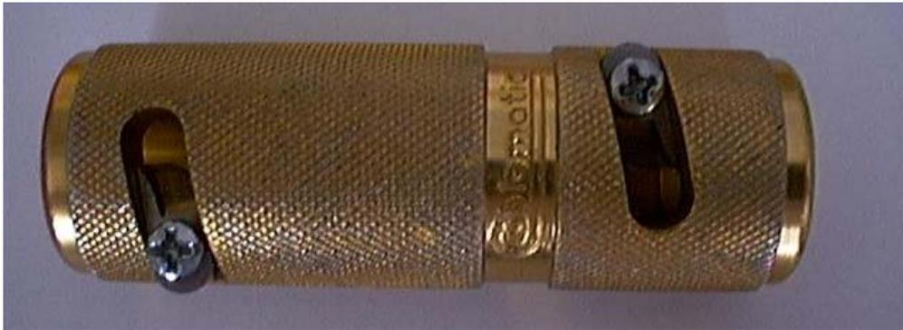
Incidentally, the center conductor SHOULD NOT stick out of the end of the PL259 once it is installed, but just shy of the end (see picture below). This is the correct length! The "Second Cut" end of the tool removes just the outer jacket to the correct length, 5/8". Other companies make coax prep tools, but this one is the best. I've had mine 25 years and it has saved me countless hours in the mean time.
