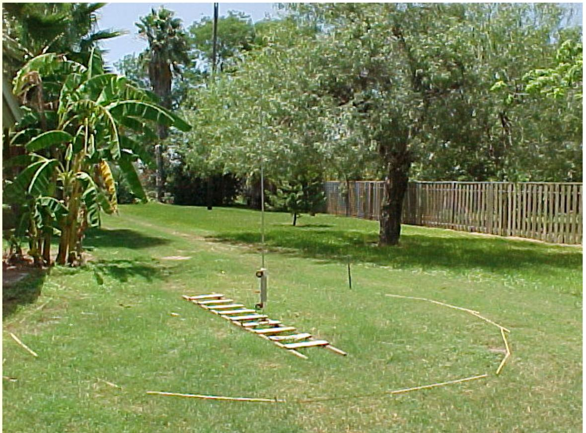
W9UCW's setup with radial field (60), base loaded vertical with RF thermocouple ammeters inserted at the top and bottom of the coil.
