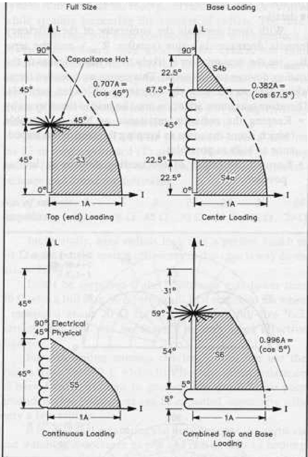
**Fig 9-40—Short loaded verticals with their current distribution. The radiation resistance is proportional to the area under the current-distribution curve. The efficiency is also proportional to the radiation resistance. See text for details.**
