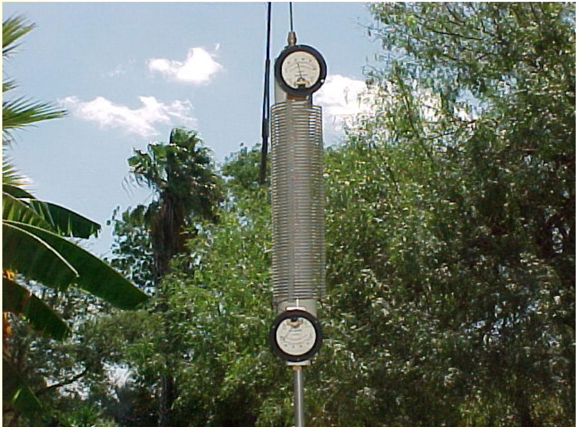
Here is the coil in center loaded radiator, 100 mA meters at both ends of the coil. The bottom one is showing full deflection (with power adjusted to) - 100 mA while at the same time the top ammeter is showing 45 mA as described above. The meters were mounted that way so that they could do a test and then just turn the coil assembly upside down and do another test to make sure results were the same and that no anomalies crept in. Results were always identical.
