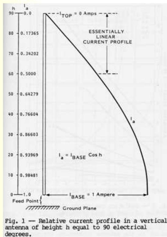
This is a true representation and shows the last 30 degrees "linearized", which is OK for simplification, but it introduces an error, which could magnify in precise calculations and modeling.
