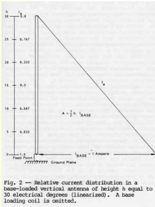
The base coil is omitted, which "simplifies" or distorts the picture of real current distribution in shortened radiator with base loading coil. As we will see later, if the coil was shown, 1 A current applied at the bottom, and current measured at the top of the coil, authors would have seen the drop across the coil and current at the bottom of the radiator (top of coil) would not be 1 A, but more like shown by the shaded area in Fig. 3.
