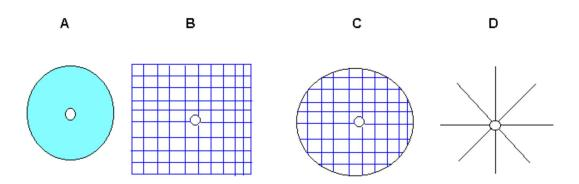
Examples of top hats are a solid disk, a square or rectangular piece of hardware cloth, a piece of hardware cloth cut in the shape of a circle, or for more capacitance, a cone, and a set of spokes. These can be straight out or bent at an angle. There should be a minimum Of three spokes. The more you use, within practical limits, the more performance the antenna will exhibit.
