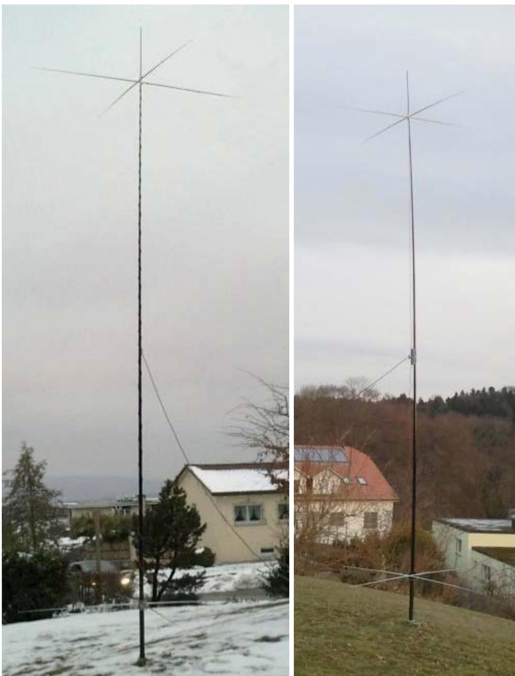
Vertical dipole for 20m (no coils) and 40m (w. loading coils), 4.8 m tall.
