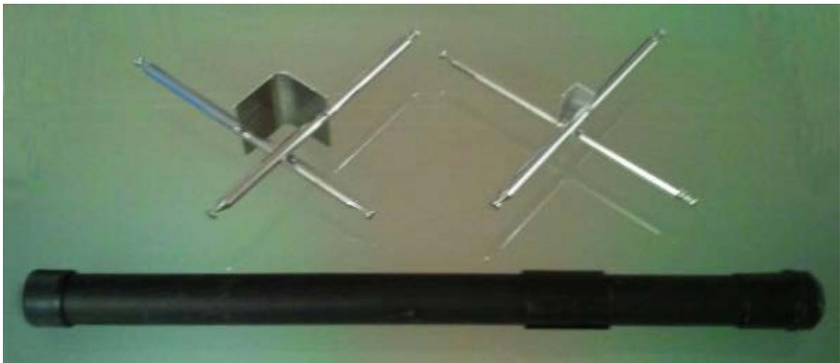
4 telescopic whips per capacity hat, total span 1.9m, mounted crosswise bottom to bottom on angle brackets of different sizes to fit the pole
