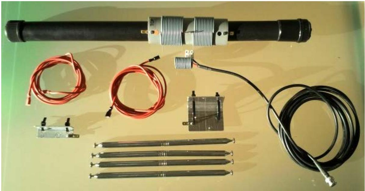
Vertical dipole for 40m, all parts, total weight less than 1.5 kg ( 3.3 pounds).
