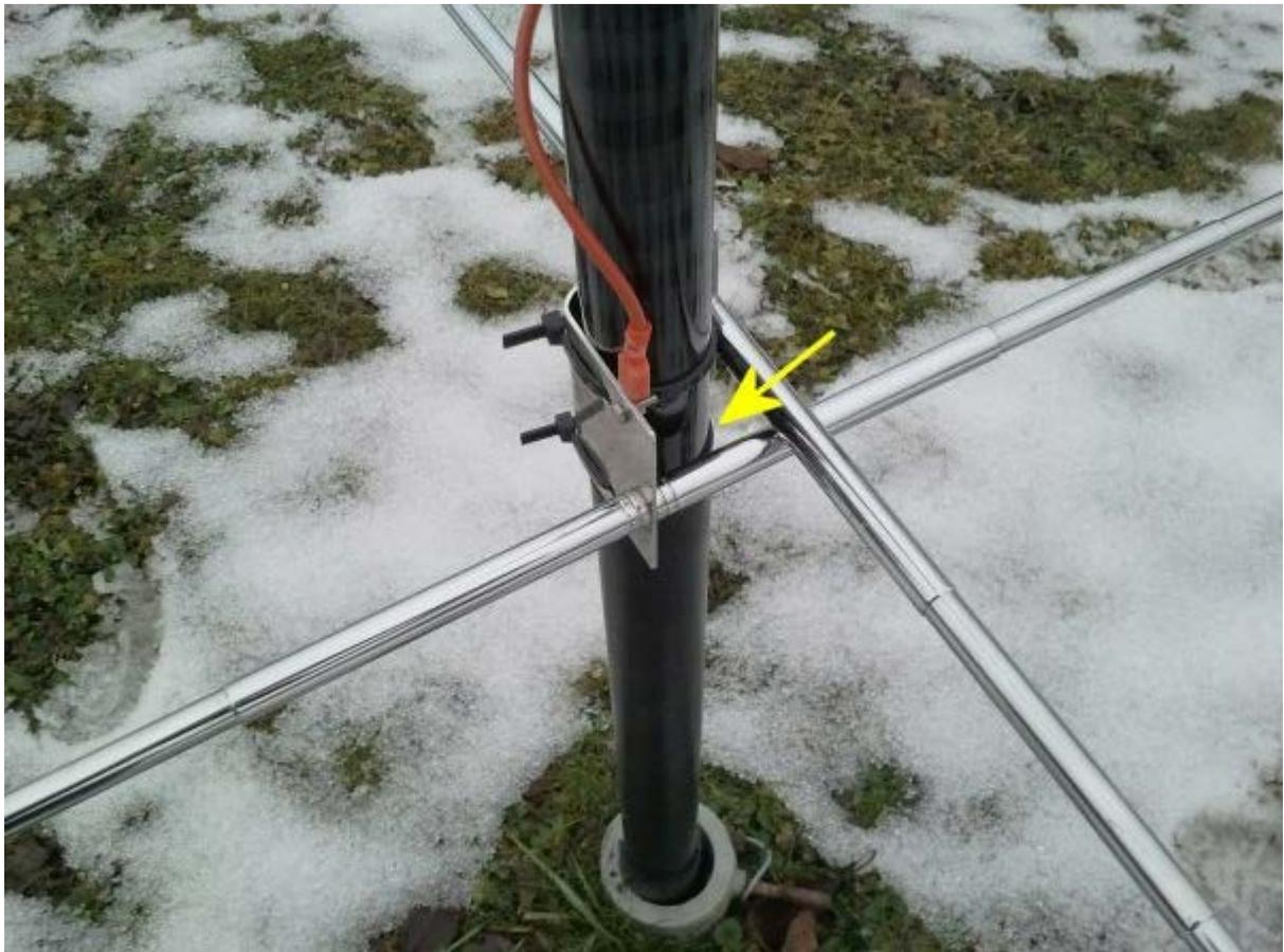
Lower capacity hat, tied to the fibreglass pole. The step between the tapered elements (yellow arrow) prevents the bracket from slipping down.
