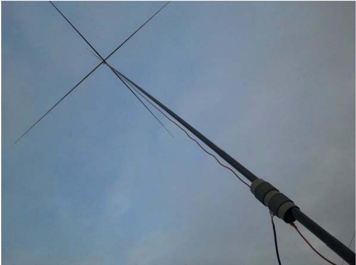
Vertical dipole for 40m, top capacity hat, loading coils and feedline.
