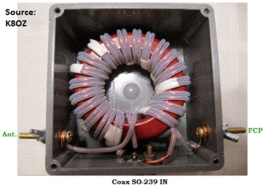
Pictured left, K8OZ's isolation transformer in the NCJ article clearly shows the correct polarity connections with marked aerial wire and FCP connections. In 2010 Jim would not have received any instruction to that effect, other than W0UCE's drawing. Likewise K9JWV's earlier drawing of the winding on a core necessarily had the same origins.
