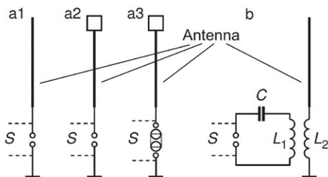
**Figure 10.** Spark gap transmitters: a) Primal Marconi transmitters with 1) only spark gap, 2) plate, 3) plate and Righi oscillator; b) Braun's coupled transmitter arrangement, after<sup>49</sup>.
