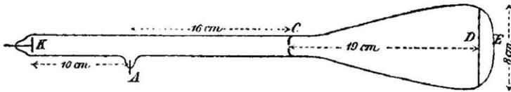
**Figure 4.** Schematic drawing of Braun’s tube<sup>35</sup>.
