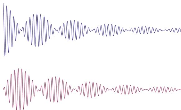
**Figure 12.** Time dependence of the currents in Braun's coupled transmitter – capacitor circuit (upper trace), antenna circuit (lower trace), after<sup>53</sup>.
