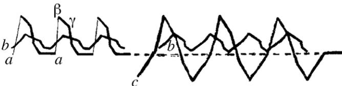
**Figure 7.** Measured waveforms of the time dependence of the current through the primary coil of a Ruhmkorff induction coil for (a) secondary coil open circuited, (b) secondary circuit short-circuited, (c) secondary coil terminated with a capacitor<sup>39</sup>.
