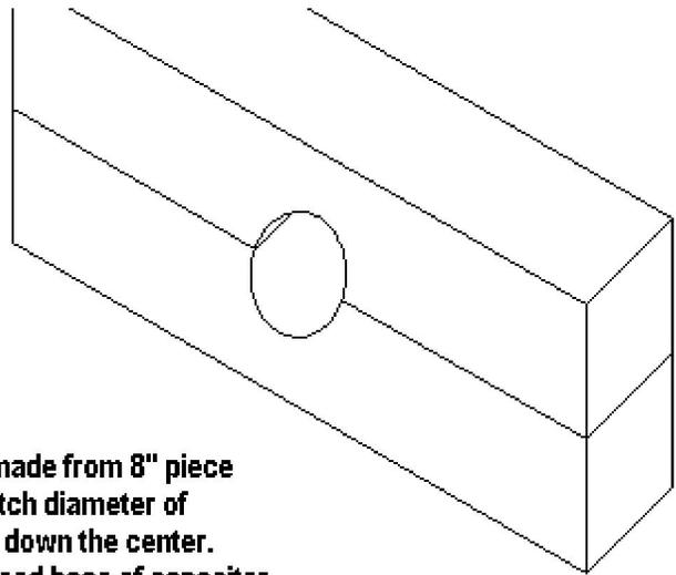
**Screwdriver hold down made from 8" piece of 2 x 4. Bore hole to match diameter of screwdriver handle. Cut down the center. Screw lower half to plywood base of capacitor assembly. Place screwdriver into cutout. Screw upper half to lower half.**
