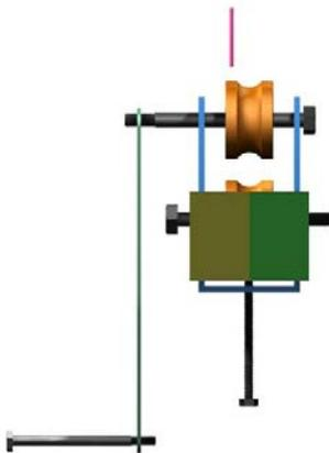
The bracket shown in blue is a building post support. Common in hardware suppliers (in Australia and New Zealand). It should be the same in your part of the world.
