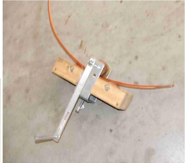
With that underway it became time to build the loop. I made the choice that I wanted a circular loop but all the information said you needed a “professional” tube rolling machine. A search of the web showed a number of home brew concepts but none seemed to allow adjustment in the range I wanted. One came close so this was designed on that.
