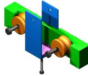
If there is a tricky piece of construction it is the driving pin for the handle roller. My pin was made from a 75mm nail. The roller is drilled right through its edge centre line. The shaft is drilled to match. The shaft is fitted to the plate and the pin gently hit flush. If it's loose, wrap the roller in PVC tape or equivalent to hold the pin in place.
