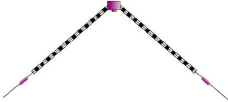
The antenna is supplied as a kit, comprising a Diamond BU-50 balun rated at up to 1.2kW, two air cored inductors wound on fibreglass formers, which function as traps on 40m and loading coils on 80m, plus lengths of 450 ohm ladder line and insulated copper wire to form the antenna elements.
