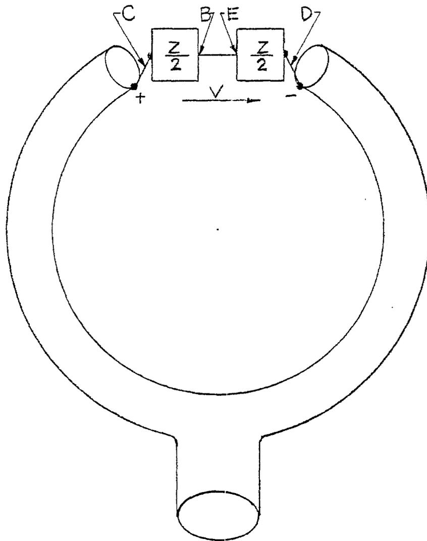
Fig. 2 Load for Split Shield Loop
