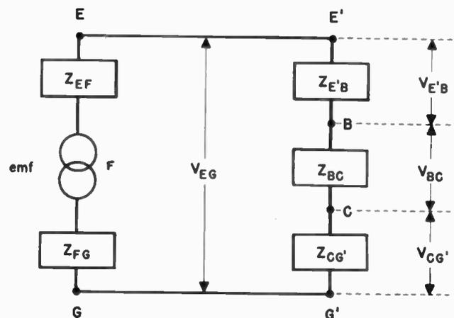
Fig. 2—Equivalent circuit of shield and gap impedances.
