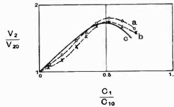
Fig. 3.—Variation of pick-up with gap loading capacitance:
