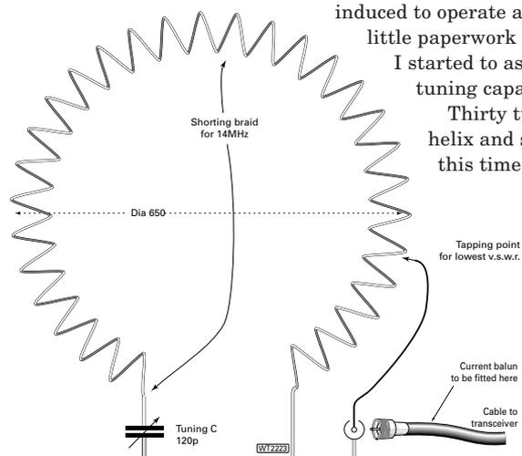
Being blessed with more than a little natural curiosity I wondered if a loop of manageable diameter and made with Slinky turns could be induced to operate as a magnetic antenna
