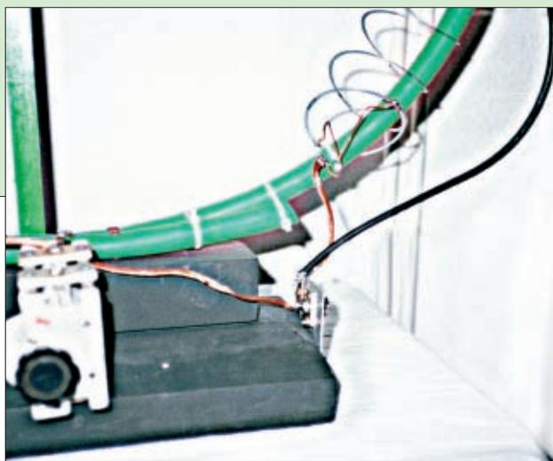
● Fig. 2: A close-up shot of the connection point, no earthing is needed for this antenna (see text for details).
