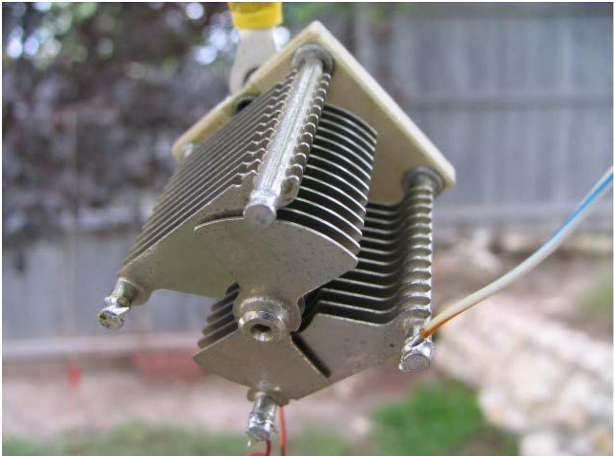
Figure 13 - Close-up of Capacitor
