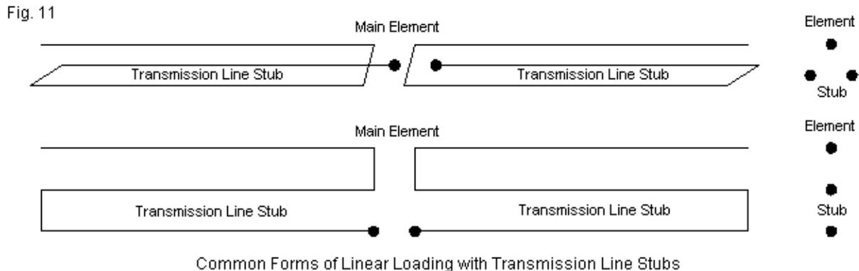
The second case that places the stubs in a linear row beneath the main element is more common to home built wire antennas than to commercial implementations of linear loading. In this scheme, the differential coupling between the two wires and the main element creates a small imbalance in the currents in the load lines. The system will still work perfectly well, but usually requires a longer stub length on each side of the feedpoint.
