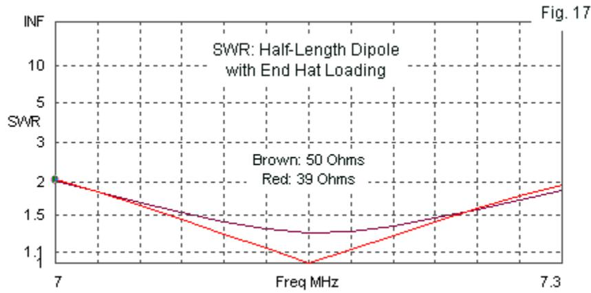
The feedpoint impedance shows a further advantage of hat loading: the SWR curve is virtually as broad as the curve for a full-length dipole. The sample antenna offers full-band coverage with less than a 2:1 50- $\Omega$  SWR even though the test-frequency impedance is a bit lower than optimal. Despite all of these advantages, the physical difficulty of implementing end hats on shortened elements tends to discourage the use of this technique, especially in the lower HF region.
