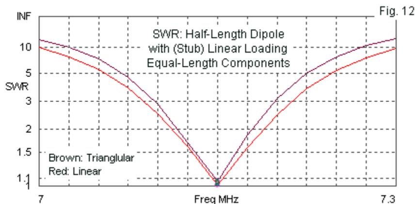
As shown in **Fig. 12**, the SWR bandwidth of a linear loaded system is only marginally broader than the curves for the center-loaded dipole with a Q or 300. The linear system is slightly broader than the triangular system, but again in the margins of significant improvement. The curves also establish the limited Q-equivalence of linear loading, since a very high Q or very low loss value for the linear loads would yield a narrower SWR operating bandwidth.
