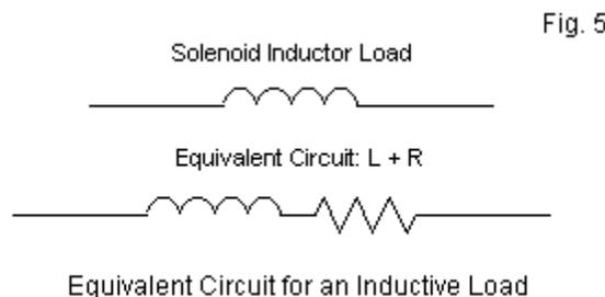
Let's begin with the center-loading coil, which has a total inductance of over 20  $\mu\text{H}$  to obtain a reactance of over 900  $\Omega$ . Practical values of Q may range from a low of 100 to perhaps 600 for a coil with a high ratio of diameter to length. Most practical coils tend to fall in the range of 250 to 350. **Table 2** shows the consequences for performance for Q values between 600 and 100 in steps of 100.
