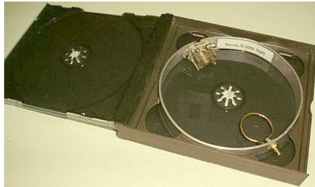
PA1AMS's test with a "CD" sized 145 MHz loop.
