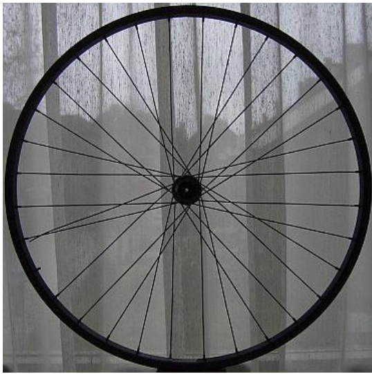
I used an aluminium cycle wheel for the loop. With a 16 - 150 pF cap the range was 11 - 30 MHz.
