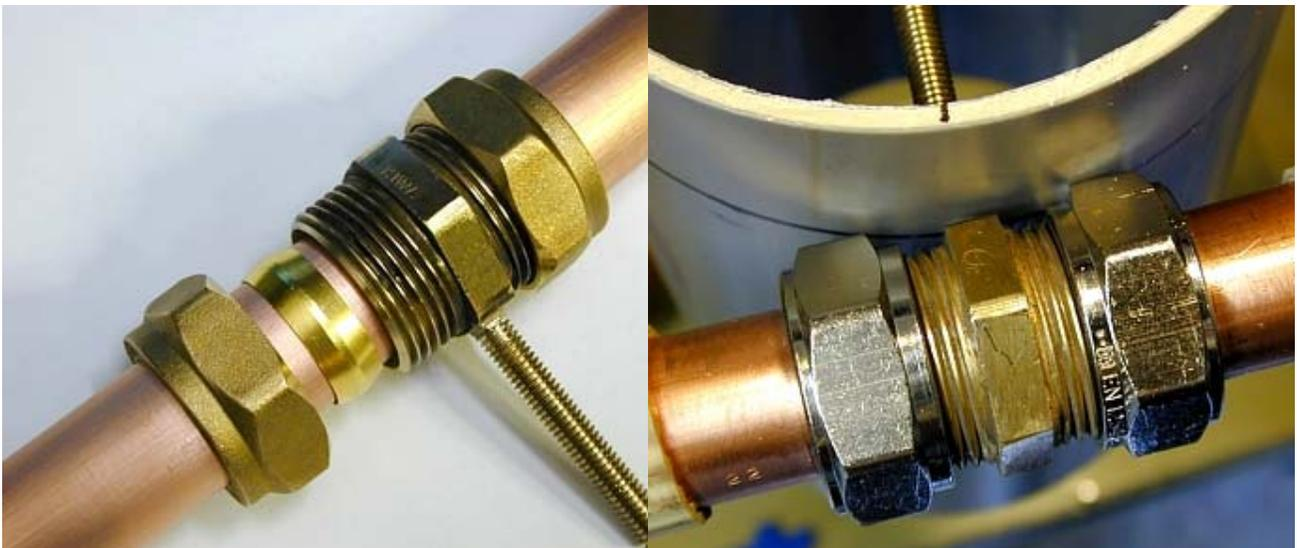
Now a key (a wrench would also work) was put to the hexagon of the coupling piece and the nuts were fixed tightly using a second key. The nuts and the hexagon differ in size and hence the key sizes should differ accordingly. Those who copy the construction should make sure that the studs of both loops will end up opposite each other (see picture).
