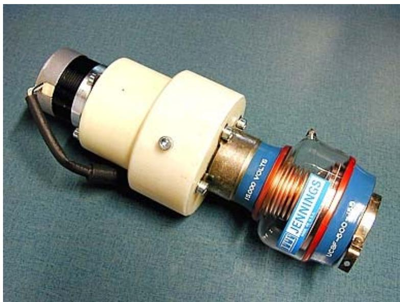
Using an ordinary variable capacitor is also possible if the plate distance is sufficiently large to accommodate the high voltages across the capacitor. Preferably use a split-stator type because of the high currents that may develop. Because of the construction of the coupling ends, positioning of such a capacitor is a rather simple matter. The studs are simply positioned downwards and thus can conveniently accommodate the capacitor (see picture).
