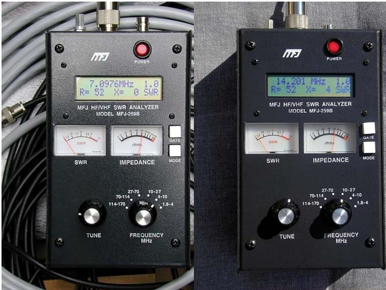
This eight-shaped magnetic loop, made from two lengths of tube of 3.70 m and 22 mm tube diameter resonated at 7.0976 MHz and 14.201 MHz with an SWR of 1:1.0 and an impedance at the feed point of at least 52  $\Omega$ . These two tube lengths are actually a bit too short to be used with 7 MHz but this was all I had and I really wanted to be able to work on this band. Surprisingly after the first CQ, CQ I immediately got a response.
