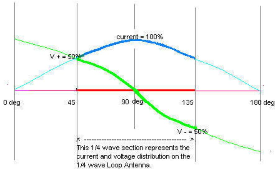
The capacitance that existed between the end sections were removed and will have to be replaced if the loop is to remain resonant and also for the current maximum to stay at the centre portion of the wire. This is achieved by placing a variable capacitor between the ends of the loop.
