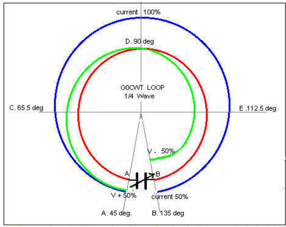
As can be seen in the drawing above I have marked out this example in electrical degrees this is because it makes it easier to relate to the original 1/2 wave dipole.
