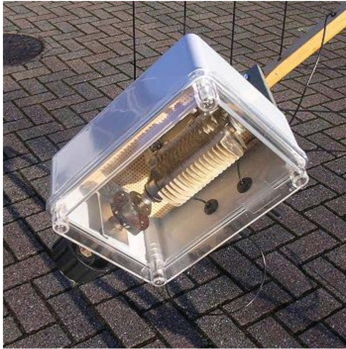
Showing the high voltage capacitor with reduction drive and waterproof enclosure. The loop connections go in at the bottom of the box through long sleeve rubber gromets.
