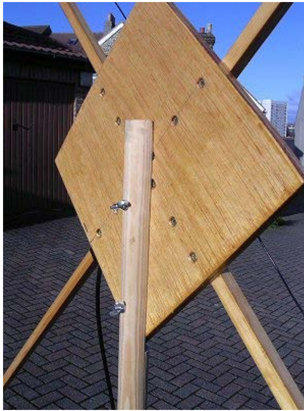
The central support showing the butterfly nut fixing to the tripod mast.
