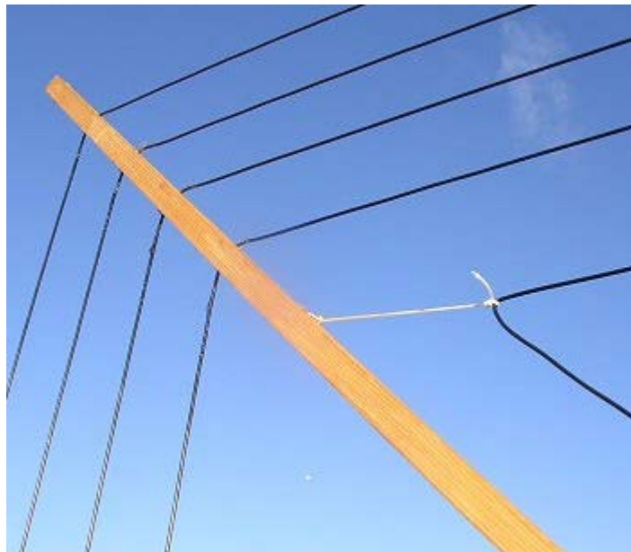
Showing a corner of the loop and also part of the coupling coil positioned using nylon cord. The wires are feed through holes drilled in the four spreader arms.
