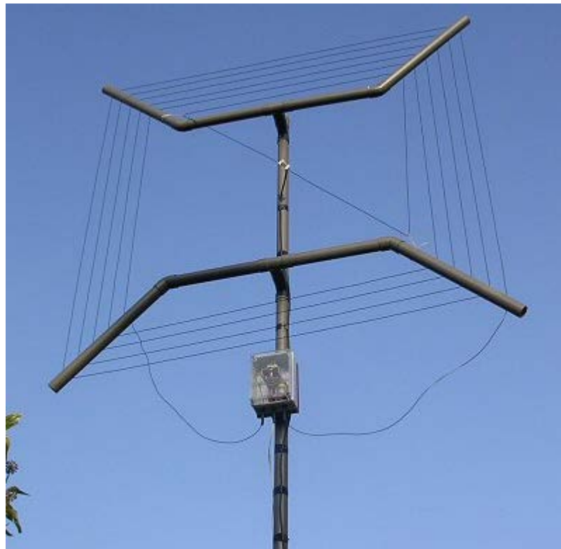
The central support showing the butterfly nut fixing to the tripod mast.
