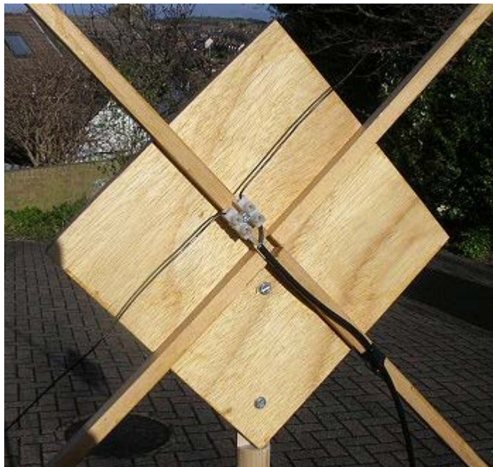
Connection of the 50 ohm coax to the triangular coupling coil.
