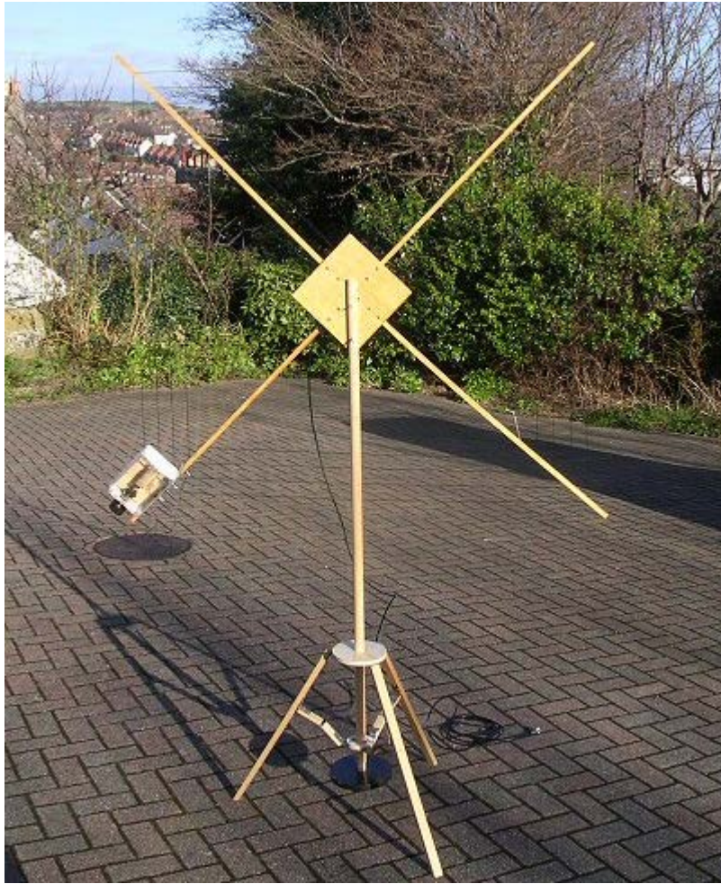
The completed copy of the frame antenna. It sits on a weighted tripod and can easily be rotated for null.
