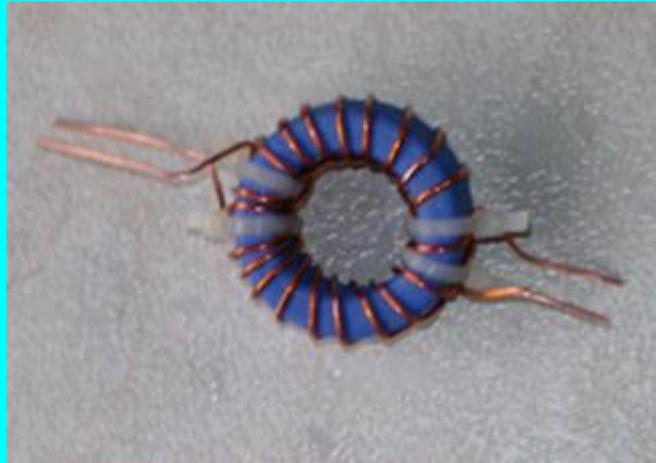
Figure 2: Voltage balun with a 1 : 1 transformer ratio
