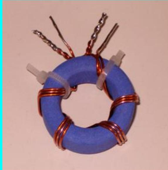
Figure 7. Trifilar 1 : 1 voltage transformer
