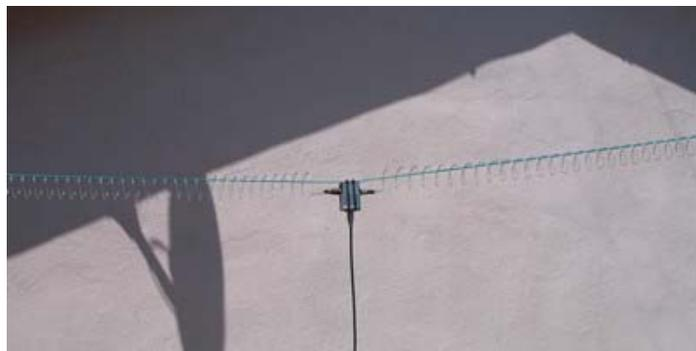
A longer range view showing a nearly 40-meter configuration. In this shot the coils are stretched out about 8 feet in either direction and held in place with alligator clips attached to the messenger line. In the final version there will a lighter cord attached to the end of each coil so the length can be adjusted at will.
