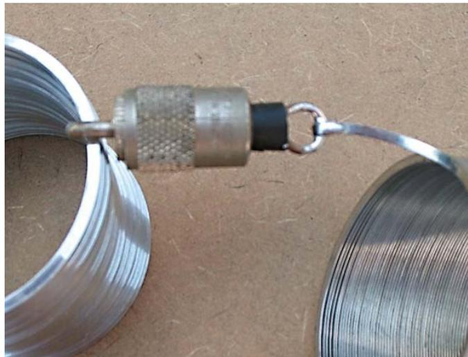
This photo shows the detail of connecting the Slinky to the loop of wire. Cut the end off the Slinky at the clip and bend a hook in it with a pair of thin nosed pliers. Hook it into the loop of wire and crimp it down with the pliers. Apply lots of solder and you're all set.
