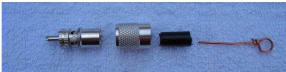
Here's how to make the end connector. Just a loop of #10 copper wire soldered into the PL-259. A small scrap of coax jacket keeps the wire from contacting the shell of the connector. It probably would not matter if it did because the connectors are not grounded anywhere. The center of the feedline goes to the center of one SO-238 and the braid of the feedline goes to the center of the other SO-238. Being mounted on plastic, the body of the connector just "floats" electrically.
