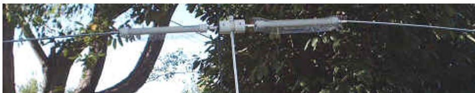
Here's a portable, dual PAC-12 dipole made with Slinky loading coils
