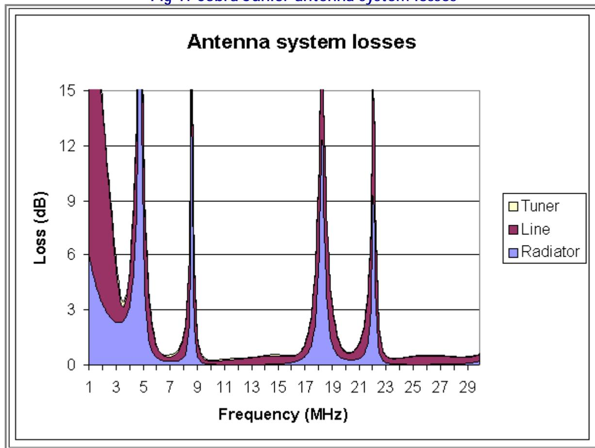
The radiator loss is quite interesting, it is very different to what would be expected from an unloaded centre fed dipole. There are peaks in radiator loss at several frequencies, and the loss in the region of these peaks is very large and would for most purposes be regarded as unacceptable.
