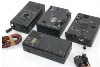
The crystal-driven transmitter (RT-6) covers 3-16MHz, divided over 2 ranges (3-7MHz and 7-16.5MHz) with a maximum power output of 10W. It has a built-in keying relay that can be used up to 40wpm (words per minute) when operating the internal key or an externally connected key. When used with an automated keyer, the cathodes of the valves would be driven directly, allowing speeds up to 60wpm.
