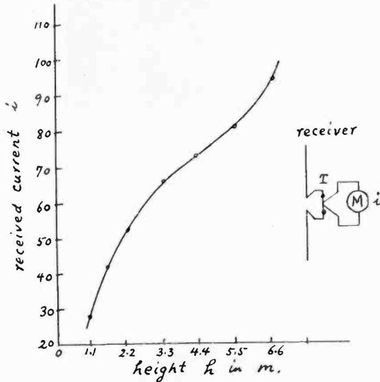
Fig. 8—The Effect of Varying Sending and Receiving Antenna Simultaneously When Wave Canal Is Located between Two Antennas.
