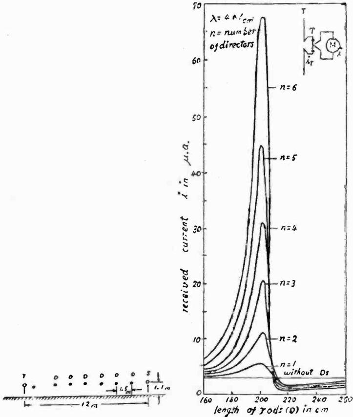
The Effect of Varying Number and Length of Directors in Wave Canals on Received Current.
