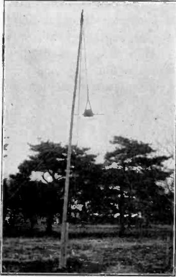
Fig. 9—Horizontally Polarized Wave Receiver in the Air.
