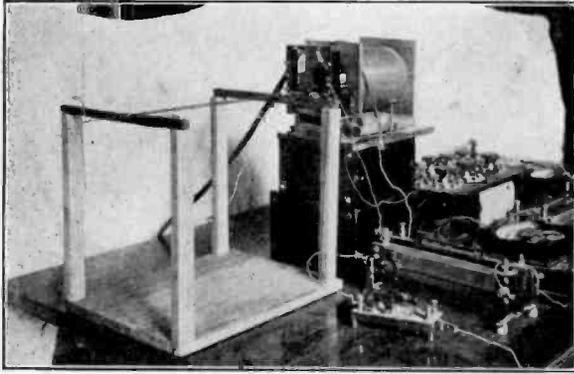
Fig. 24—Apparatus for 26.5-150 cm. Wavelength Production.
