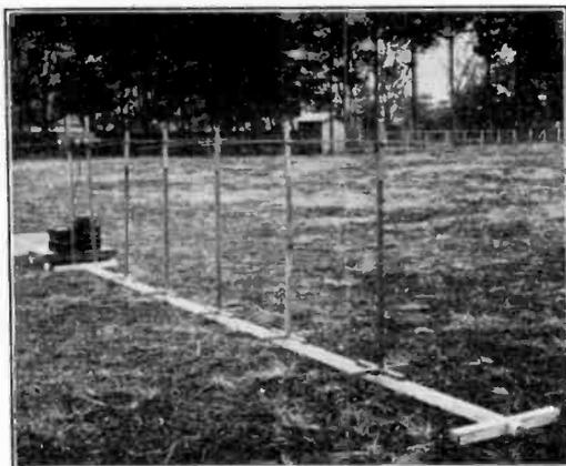
Fig. 19—Projector Horizontally Polarized Wave; 260 cm.
