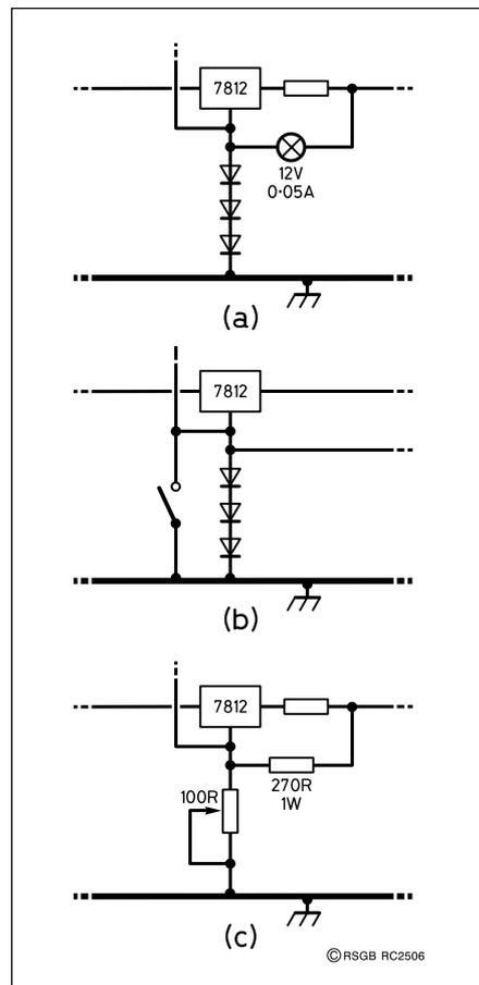
Fig 7: Alternative methods of providing 13.8V output (b) with switch closed for 12V.
