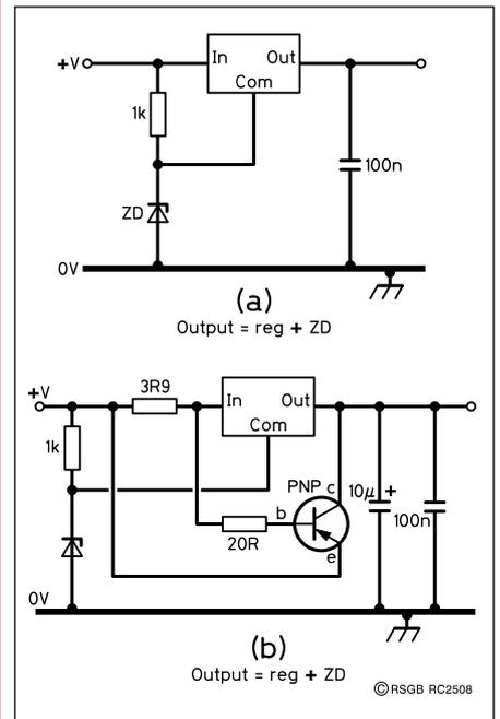
Fig 9: (a) Use of a Zener diode to increase the regulated voltage. (b) For high currents, a suitable series bypass transistor (with heat sinking) may be used.
