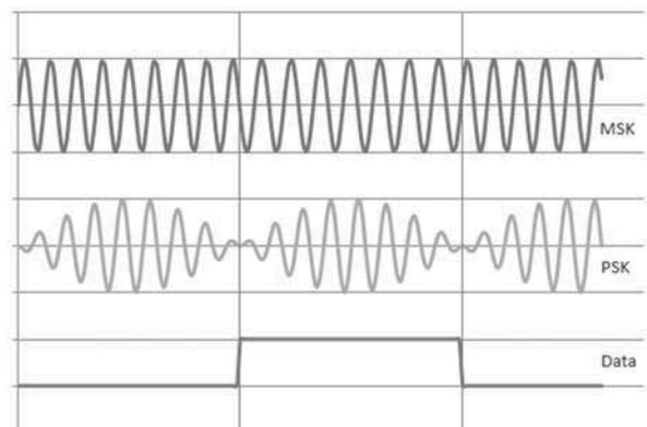
Figure 3. Illustration of PSK and MSK modulation.
