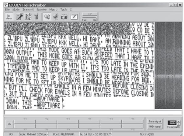
Figure 2. VK2DDI receiving ZL1BPU on 508.1 kHz using IZ8BLY Hellschreiber.
