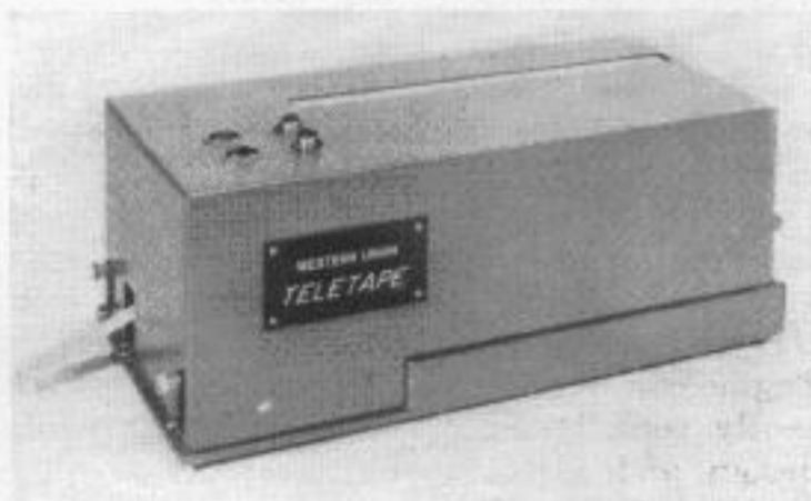
Figure 9. Transceiver with self-contained amplifier and control unit
