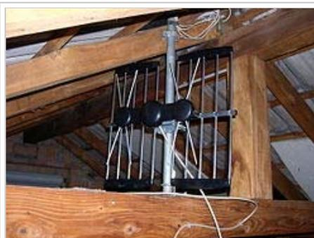
A modern form of reflective array is the "bow tie" UHF television antenna. This example has two dipole driven elements in front of a grill reflector oriented for vertical polarization. The "bow-tie" dipoles, consisting of two V-shaped elements, have a larger bandwidth, allowing the antenna to cover the wide UHF television band.
