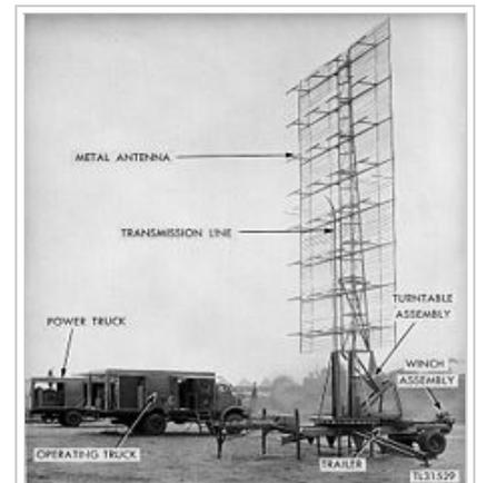
Reflective array 'billboard' antenna of the AN-270 radar, an early radar system used in 1941 at Pearl Harbor. It consists of 32 horizontal half wave dipoles mounted in front of a 55 ft. high screen reflector. With an operating frequency of 106 MHz and a wavelength of 3 meters this large antenna was required to generate a sufficiently narrow beamwidth to locate enemy aircraft.
