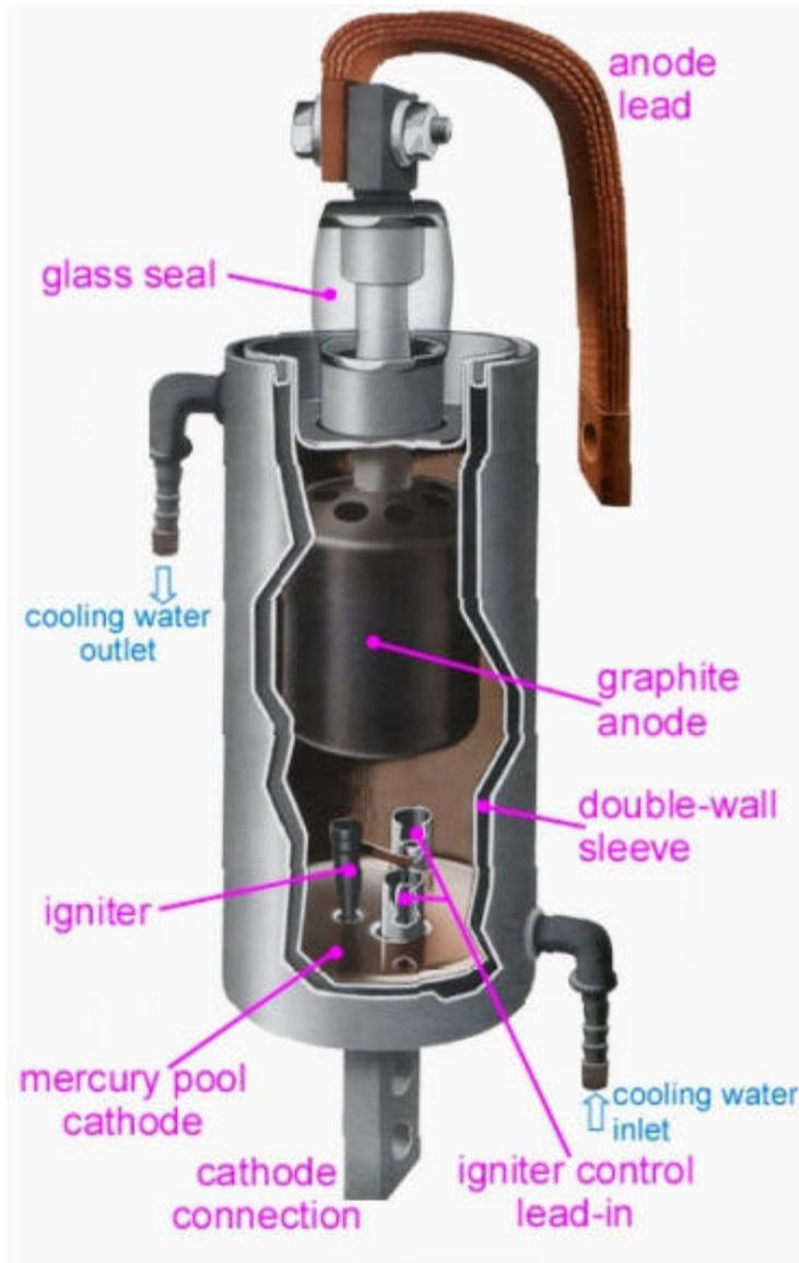
**Cut-away view of a basic ignitron**
