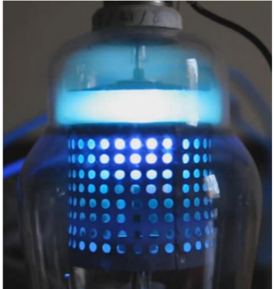
***Cut-away view of the electrode arrangement of a thyatron***
