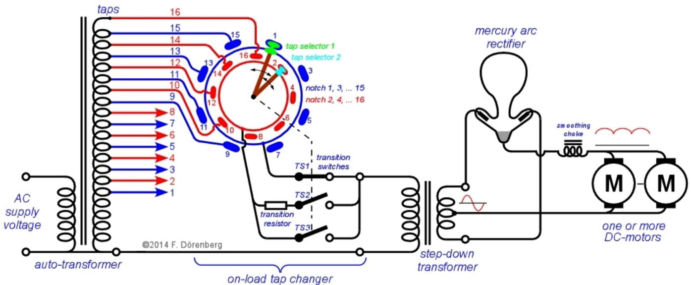
**Figure 2: Principle of DC-motor speed control with an On-Load Tap Changer and full-wave Mercury Arc Rectifier**
