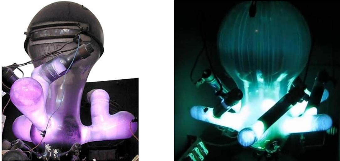
*Figure 1: 3-anode and 6-anode Mercury Arc Rectifier*
