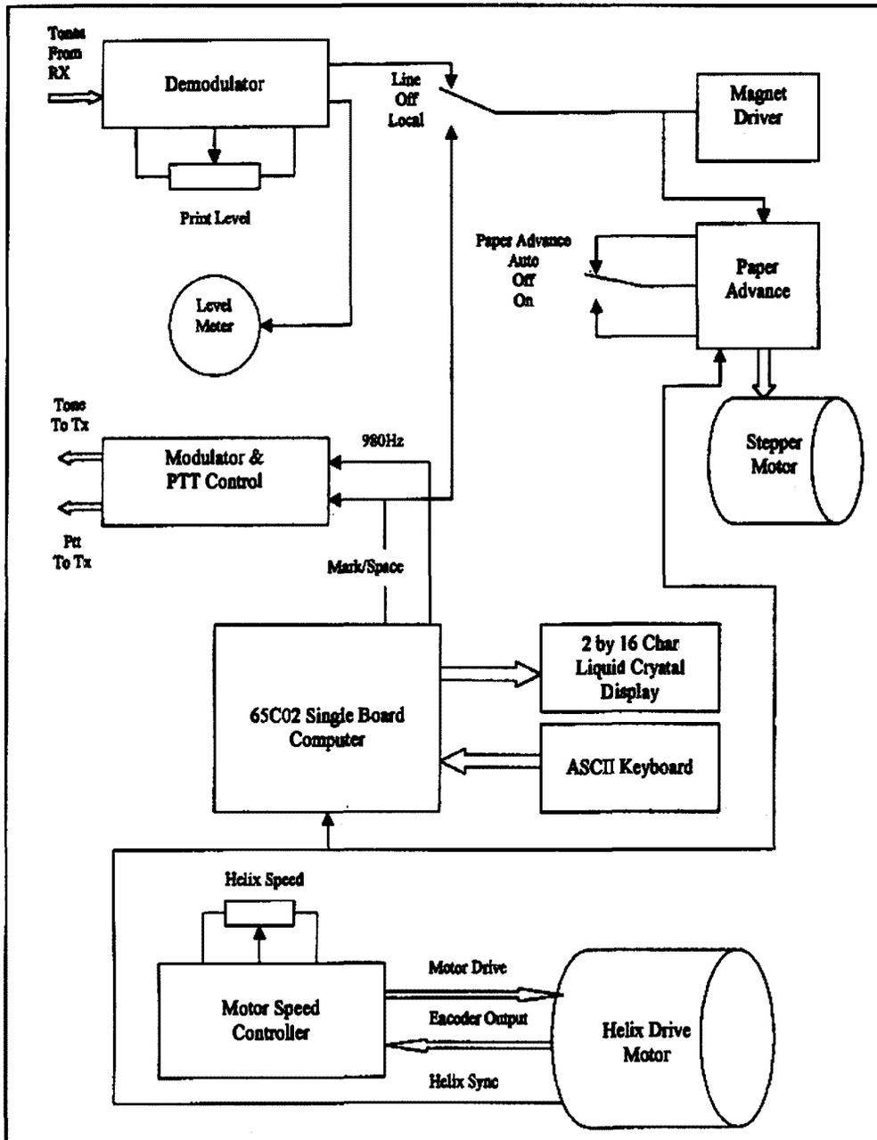
Figure 9: System block diagram.
