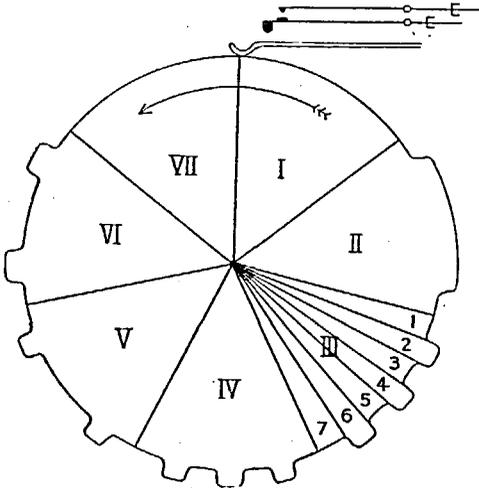
Fig. 3.—Diagram of cam disc for producing a letter E impulse train
