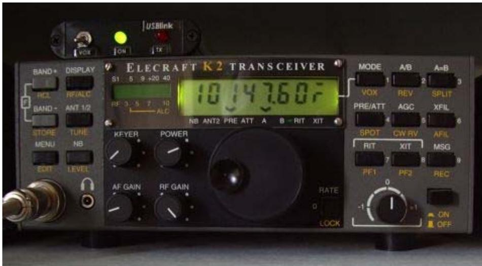
I made up interface cables for both my FT-817ND and Elecraft K2 and have tested the USBlink with both radios. Several QRP PSK31 contacts were successfully made and the USBlink is now in full time use in my HF packet radio APRS station.
