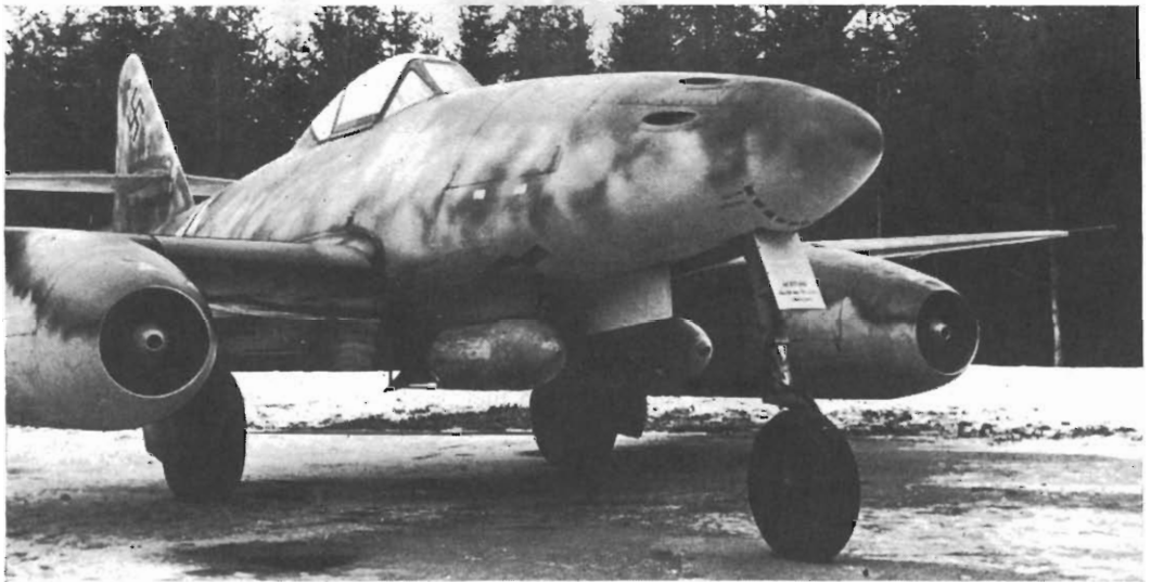
(Above and right) An Me 262A-2a Werk-Nr. 110 813 with two 551-lb. SC 250 bombs. This fighter-bomber variant, which first entered service with a detachment of KG 51 commanded by Major Wolfgang Schenck during the summer of 1944, differed from the standard fighter solely in having pylons and bomb-fusing equipment.
