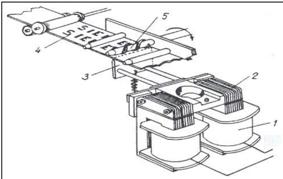
1 printer magnet; 2 iron core; 3 paper guides; 4 paper strips; 5 printer spindle threads;
