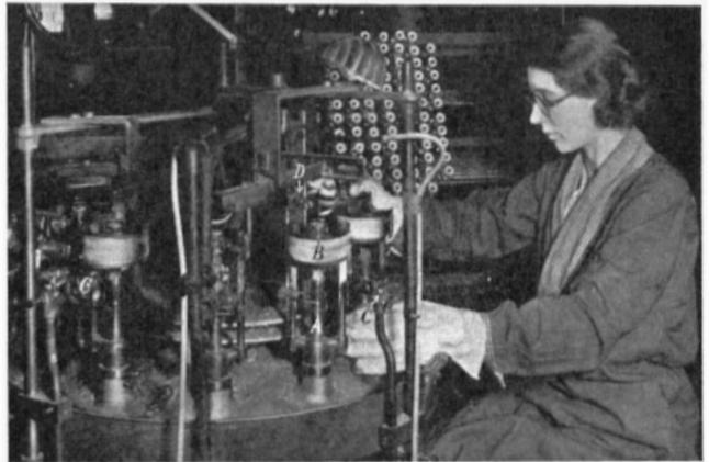
Fig. 7. Sealing-in machine
