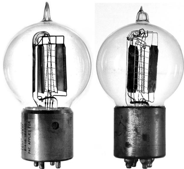
**Fig. 9.** The tube on the left hand side is the first designed by van der Bijl (type M or 101A). On the right is an improved version (type L or 101B with double inverted V filament). These were the tubes used on the transcontinental telephone line in 1914. The M stood for mounted (in these prototypes the base was made from machined brass) and the L stood for line. Tubes in SAIEE collection; photo by the author.
