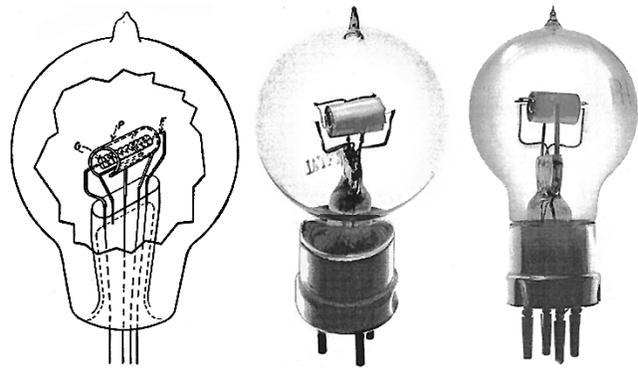
**Fig. 11.** On the left is a sketch of "a tube of simple construction" designed and produced by van der Bijl in September 1914. He claims that this was the origin of the French TM tube, an example of which is shown in the center. The British *R* valve shown on the right was based on the TM. Many millions of these tubes were made during and after World War I. Tubes in SAIEE collection; photo by the author.
