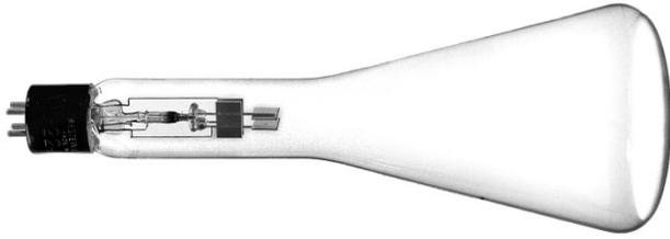
**Fig. 14.** Van der Bijl suggested gas focusing these early cathode ray tubes intended for use in oscilloscopes. Tube in SAIEE collection, photo by the author.
